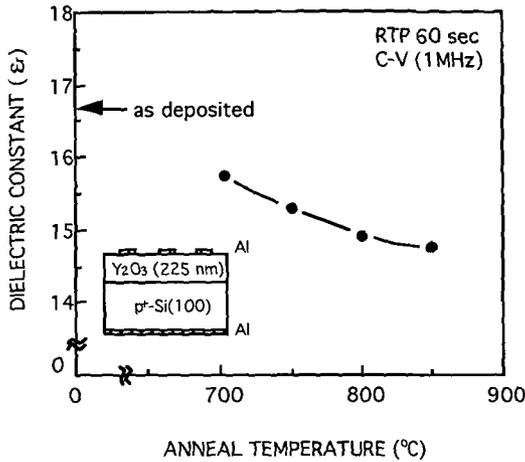
Fig. 3 Dielectric constant  $\epsilon_r$  of  $Y_2O_3$  as a function of RTP-treated temperature. Arrow indicates the  $\epsilon_r$  value of the as-deposited film.
