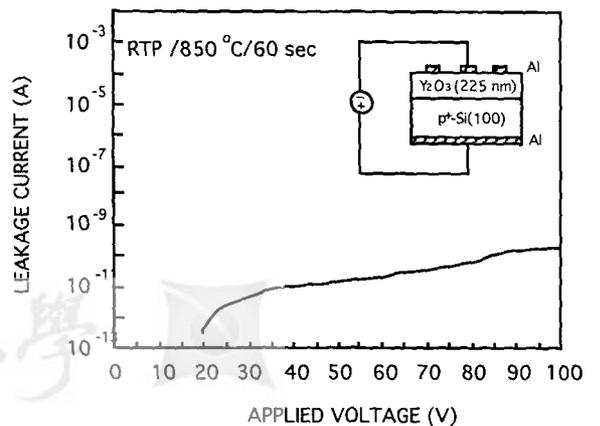
Fig. 5 Current-voltage relationship for a  $Y_2O_3$  film after RTP for 60 sec at  $850^\circ C$ .
