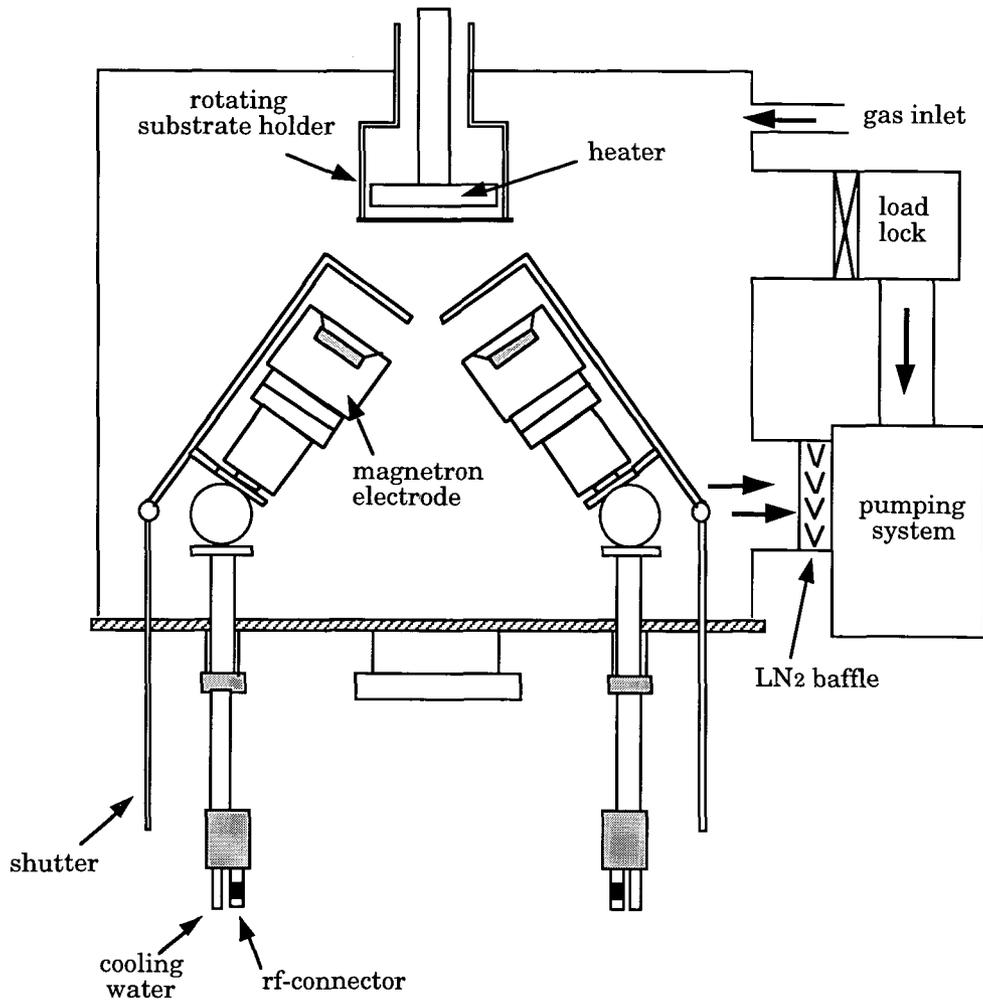
Fig. 1 Schematic diagram of the sputtering system used in this study. The system is equipped with in-situ tilted electrodes and a load-lock chamber.
