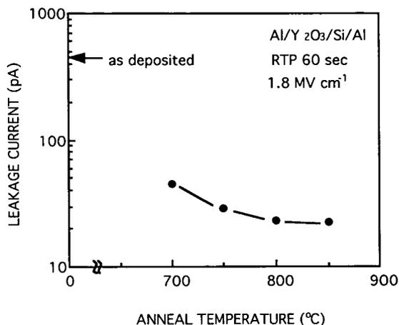
Fig. 6 Leakage current of  $Y_2O_3$  as a function of RTP temperature. Arrow indicates the leakage current of the as-deposited film.
