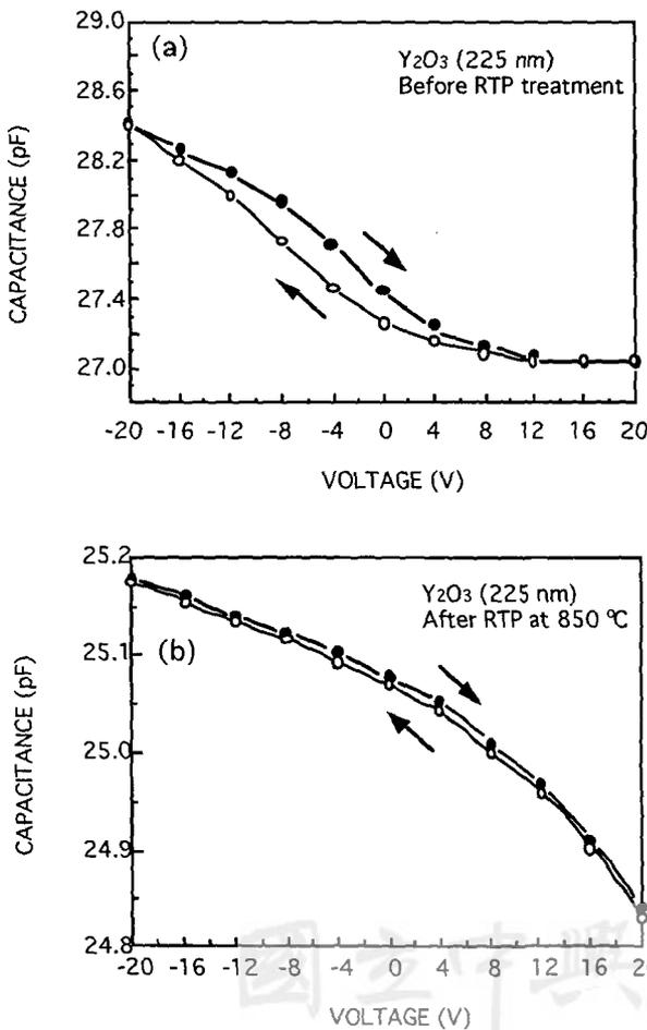
Fig. 4 Typical capacitance-voltage plots for (a) a  $Y_2O_3$  film after RTP at  $850^\circ C$  for 60 sec and (b) the as-deposited film.
