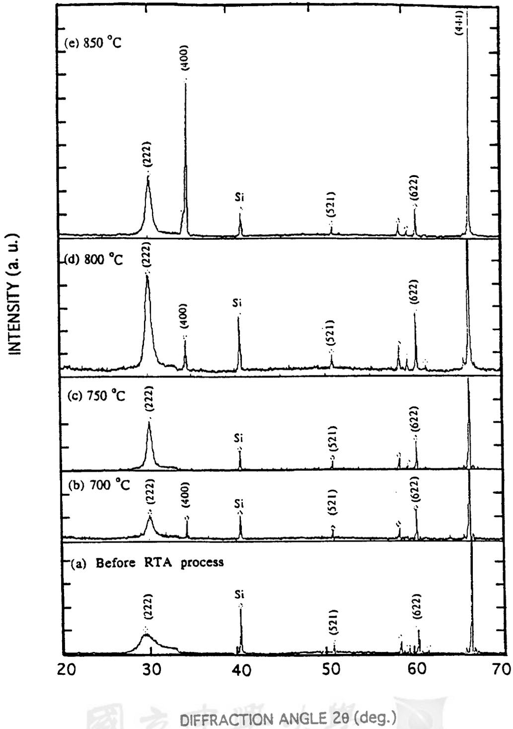
Fig. 2 X-ray diffraction patterns of  $Y_2O_3$  thin films for RTP at different temperatures as compared with that of the as-deposited film.
