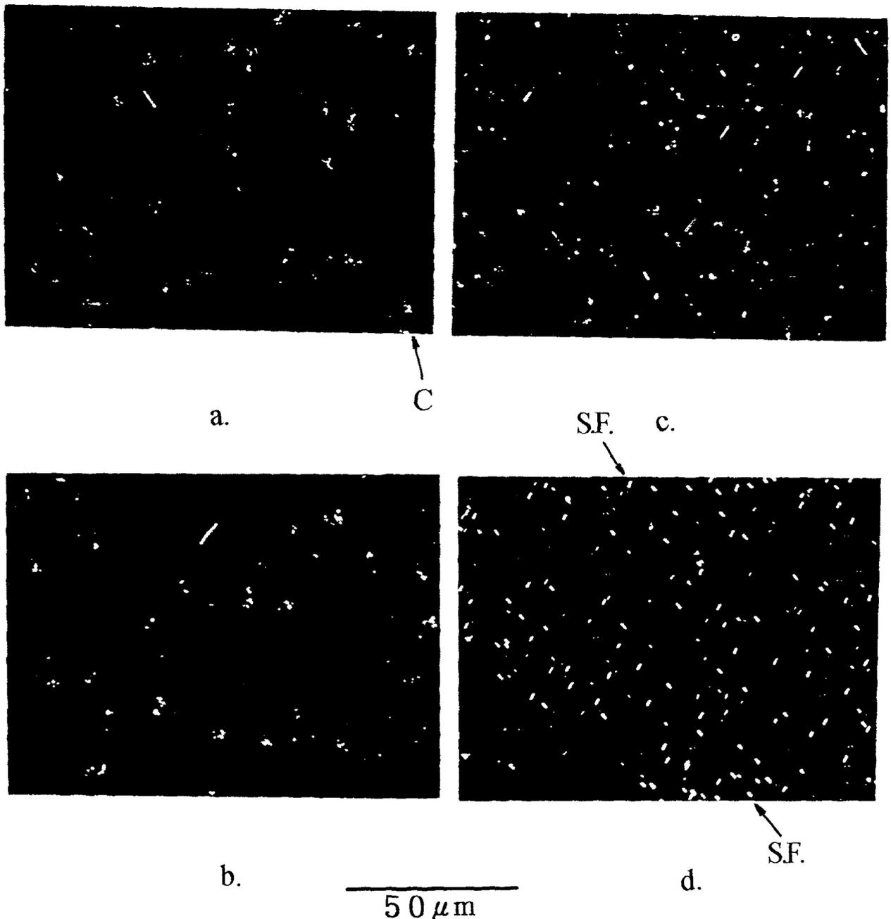
Fig. 3 Optical photomicrographs of wafer cross sections after a 40-h growth anneal at 1000°C preceded by a 1-h pre-anneal at 1150°C and nucleation annealing at 450°C for times of (a) 0 h, (b) 16 h, (c) 64 h, and (d) 128 h. Samples were Wright etched for about 3 min. to delineate the defects.
