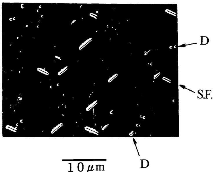
Fig. 4 A typical SEM photomicrograph of a wafer cross section after a 40-h growth anneal at 1000°C preceded by nucleation annealing for a time longer than 256 h.
