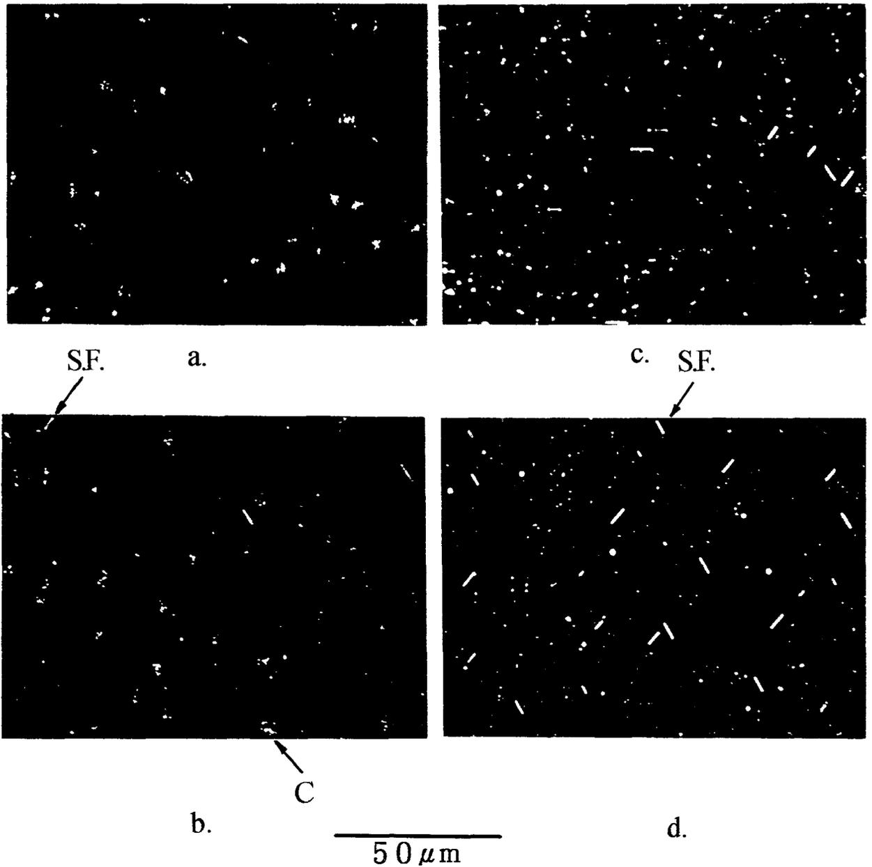
Fig. 2 Optical photomicrographs of wafer cross sections after a 40-h growth anneal at 1000°C preceded by nucleation annealing at 450°C for times of (a) 0 h, (b) 16 h, (c) 64 h, and (d) 128 h. Samples were Wright etched for about 3 min. to delineate the defects.
