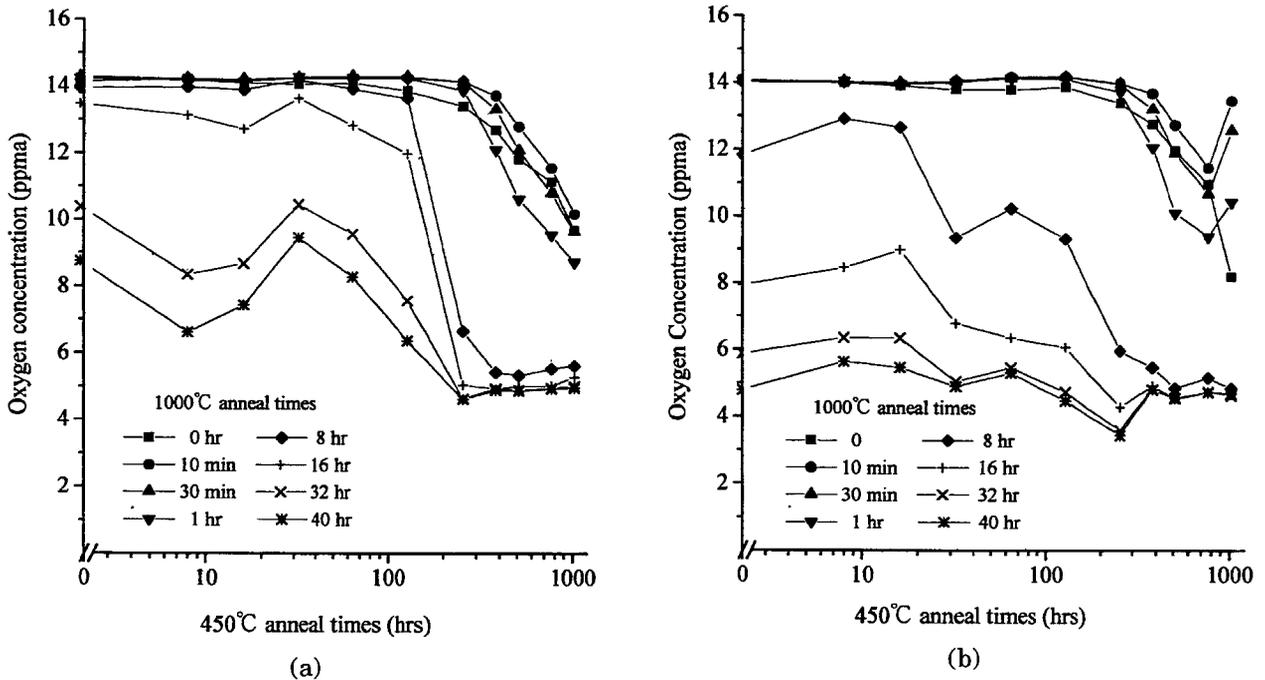
Fig. 1 Oxygen concentration after different growth anneal times at 1000°C as a function of the nucleation anneal time at 450°C. (a) Two-step process. (b) Three-step process.
